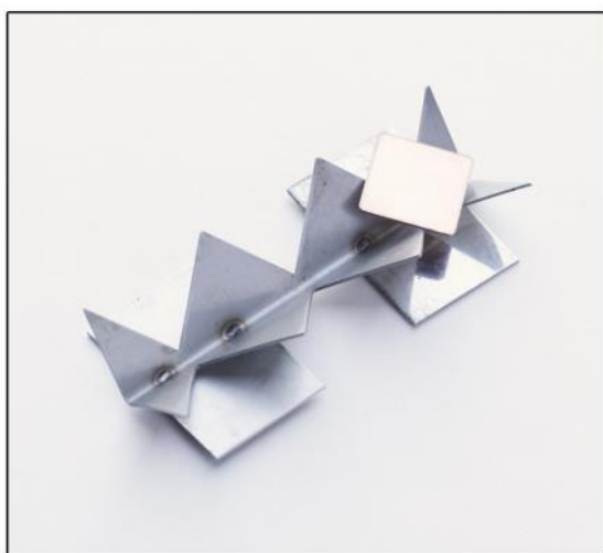
Trivet 2814 - small, stainless steel, 27mm wide span at the top of each 'V', 3 piece support 3x4 prongs. Dimensions at base 35x80mm. Shown supporting a 18mm square.
